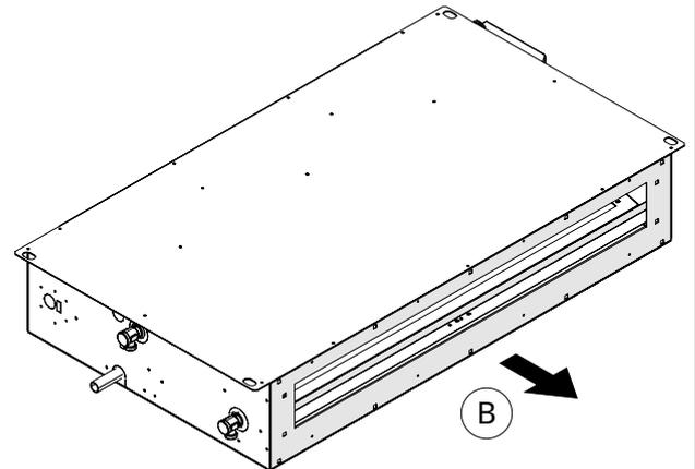
**Installation verticale****A** Reprise air ambiant**B** Refoulement air
